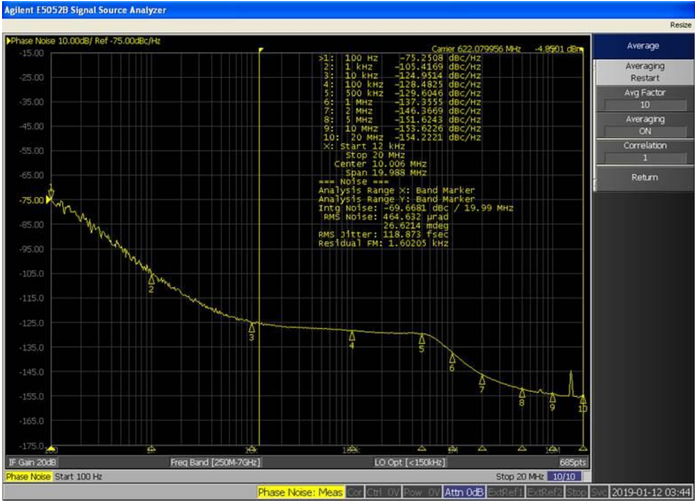
Figure 3. Representative Phase Noise Measurement: F_{OUT} = 622.08\text{ MHz} , F_{IN} = 10\text{ MHz} , BW = 100 Hz
