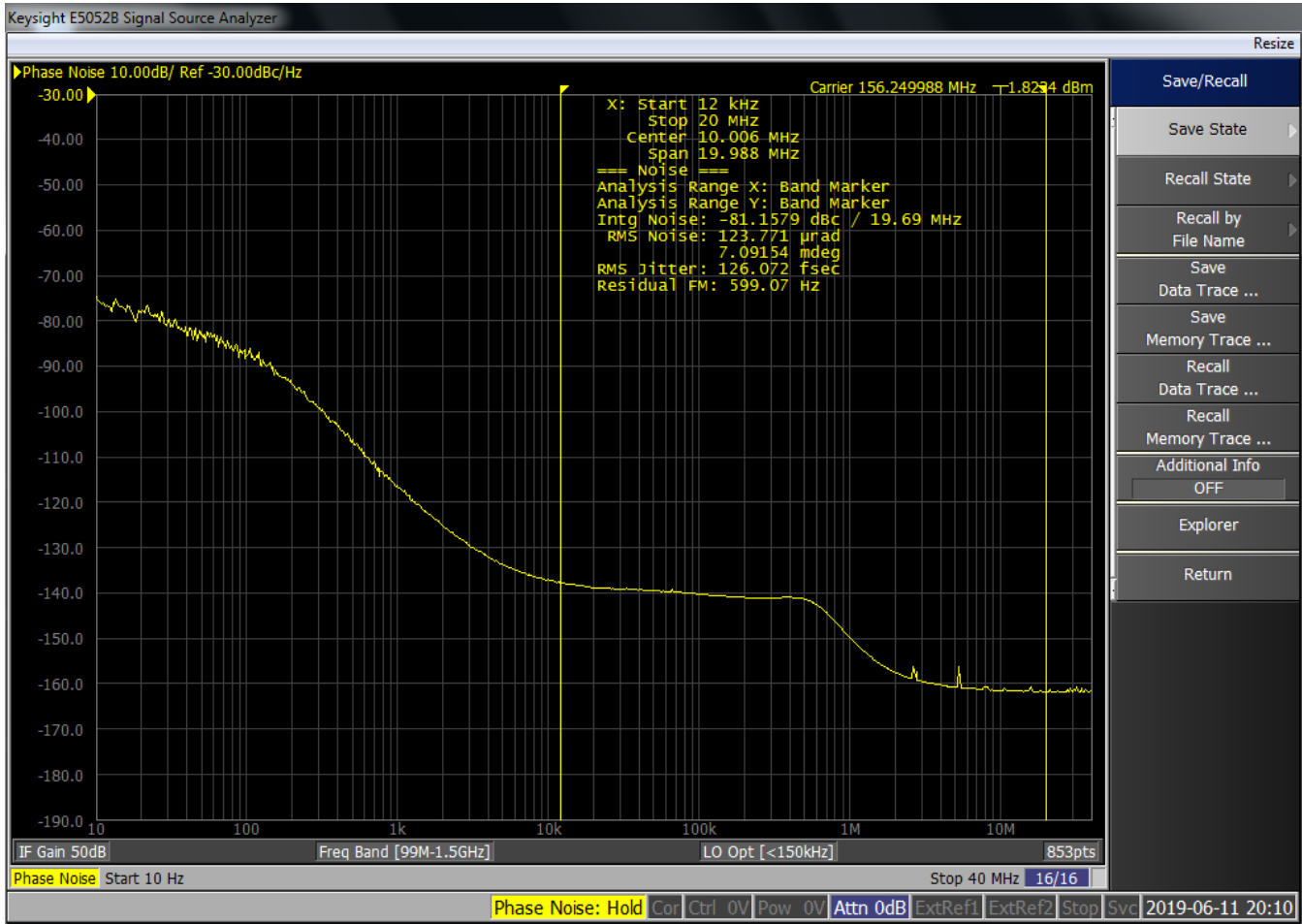
Figure 4. Representative Phase Noise Measurement: F_{OUT} = 156.25 MHz, F_{IN} = 10 MHz
